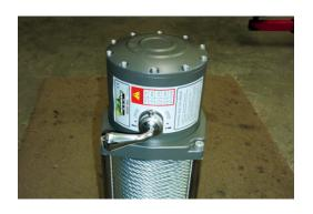
2. Undo and remove 2 chrome Allen head bolts which hold the gearbox to the tie rods.
