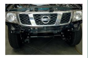
8. Once bar is aligned with vehicle and tightened, drill through pinning holes between bull bar and chassis brackets. Secure with hardware provided.
