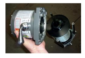
NOTE: If shaft comes out of cable drum remove it from the gearbox and place it back into the drum making sure it engages with the brake.
