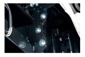
9. Fit protection plate to underneath of bull bar using M8 bolts, spring washers and flat washers provided.
