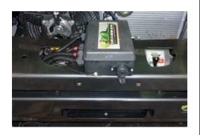
12. Connect three colour coded cables to the corresponding poles on winch motor.
