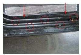
7 x Holes will need to be drilled to 12.5mm in front cross member
