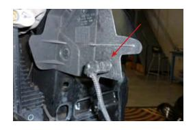
9. Place chassis bracket in position on chassis and mark location of all mounting holes onto front cross member. Remove chassis bracket and drill all holes to 12.5mm.
