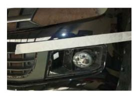
5. Using an air hack saw or similar, cut along the line previously marked to remove the lower section of the bumper.
