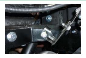
13. Refit plastic bumper reinforcement and top section of bumper bar.
