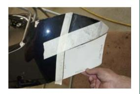
8. Remove ambient air temperature sensor and fit to plastic panel as shown.
