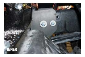
NOTE: Nut, flat washer and spring washer between bracket and crossmember.
