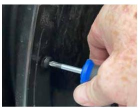
4. Prepare flare by removing a small portion of 3M protective cover. Attach masking tape as a tail for easement of fitting. Anchor the flare to its original position without tighting the screw completely, so that the flare can move and adjust into its position.
