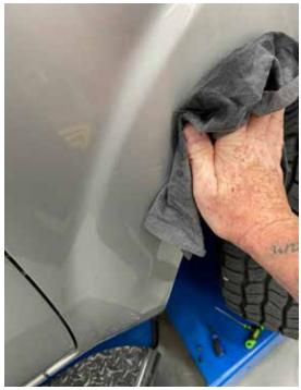
2. Start the installation on the front right flare by first placing the flare into the position to be installed. Check the position and alignment.
