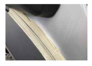
**10.** Apply a small amount of silicone sealer along the middle of the taped edge.
