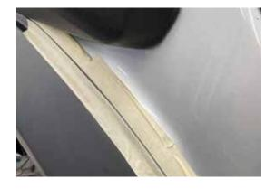
**10.** Apply a small amount of silicone sealer along the middle of the taped edge.
