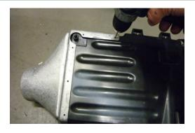
10. Secure in place using pop rivets provided.
