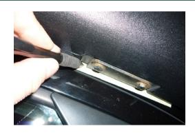
23. Hold pillar bracket in position previously marked and mark three mounting holes. Drill holes to 7.5mm.
