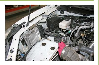
**3.** Remove front ECU and mounting bracket (A). Remove airbox retaining bracket (B).
