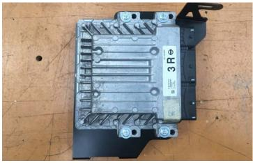
Mount ECU's into back right hand corner of engine bay using 2 x M6 bolts removed from original computer bracket. Do not fit upper bolt on the inner guard, this will be completed later.
