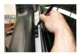
9. Drill mounting holes in pillar to 7.5mm. Apply silicone sealant. Insert mounting plugs and attach mounting bracket using three self tapping screws provided. When drilling mounting holes, only drill through outer skin and no further.
