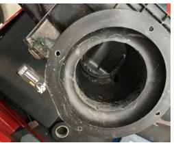
2. Using the air hacksaw or similar, cut centre section of the inner air box inlet to allow more airflow
