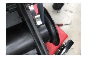
14. Add sensor safe sealant to the air box adaptor and pop rivet to air box
