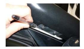
10. Hold bracket in position previously marked on pillar and mark mounting holes.
