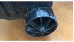
16. Refit air box for vehicle, attach to rubber joiner and attach with hose clamp provided.
