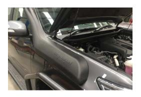
13. Attach rubber pipe to snorkel and secure with hose clamp provided.
