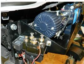
32/ Route the remote control wiring up to the hole you drilled in the front bumper.
