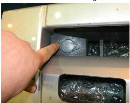
This kit and these instructions are to fit a Superwinch alloy fair lead flush with the front of the bumper. The mounting holes will be in the same place on other winches but the trimming of the bumper and the spacers may be different!
